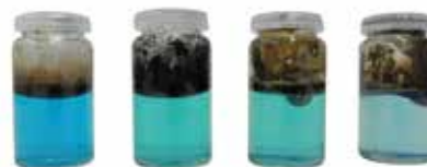
The intensity of the blue colour refers to different total iron concentration measured in Cylinder Drain Oil (CDO) samples
