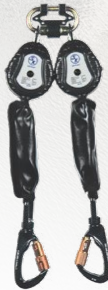
6' Webbed SRL Code: FPSKELE06D Includes Dual Carabiner and Aluminum Quarter Turn-Locking Hook
